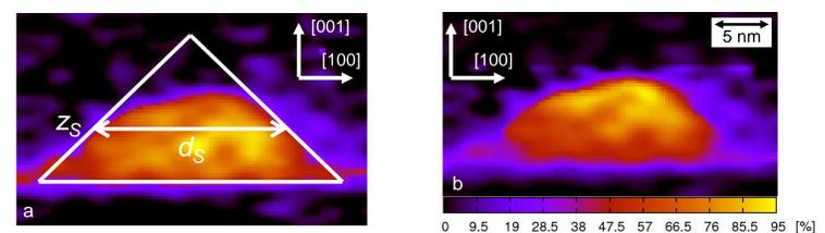
Fig. 6: a) Determination of the pyramid's parameters, b) shape corrected In-concentration
