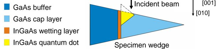
**Task:** Determination of the local extent of the QD with respect to the sample thickness along the incident beam direction to correct the CELFA result.
