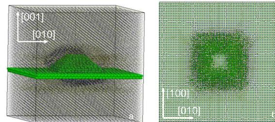
Fig. 3: a) three-dimensional view of a pyramidal QD with truncated top and {101} facets; b) plan-view sight of that model
