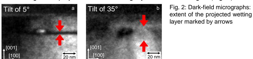
Fig. 2: Dark-field micrographs: extent of the projected wetting layer marked by arrows
