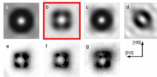
Fig. 4: simulated plan-view BF images of different QD shapes: a) sphere, b) pyramid {101}, c) pyramid {112}, d) pyramid {136} and e-g) experimental data
