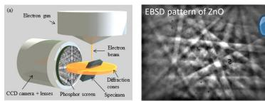
Left: Scheme of EBSD acquisition. Backscattered electrons from a highly tilted sample generate a so-called Kikuchi pattern on a phosphor screen, that is then captured by a camera (<u>https://en.wikipedia.org/wiki/Electron\_backscatter\_diffraction</u>). Right: Exemplary EBSD pattern showing Kikuchi bands from electron diffraction.
