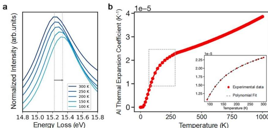
Literature example for temperature measurement using an Aluminum specimen. (a) EEL spectra of the Aluminum bulk plasmon for different temperatures showing a shift due to lattice expansion and a related change of the electron density. (b) Thermal expansion coefficient for Aluminum. [1]
