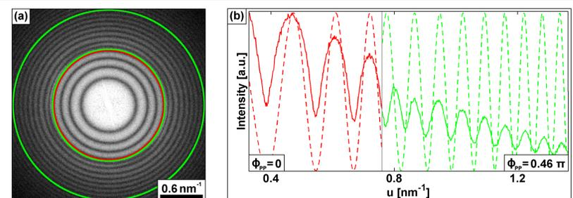
Fig. 6: Application of a PCS-film-based Zernike PP on an aC test object.
