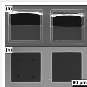
Fig. 2: Scanning electron microscopy image of a 1x2 array of (a) Hilbert PPs and (b) Zernike PPs.
