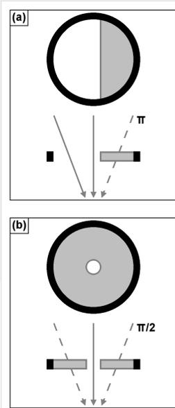
Fig. 1: Schematic illustration of a (a) Hilbert PP and (b) Zernike PP located in the back focal plane of the objective lens.
