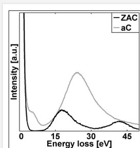
Fig. 3: EELS spectra of a 24 nm ZAC- and a 49 nm aC-film taken at 120 kV.
