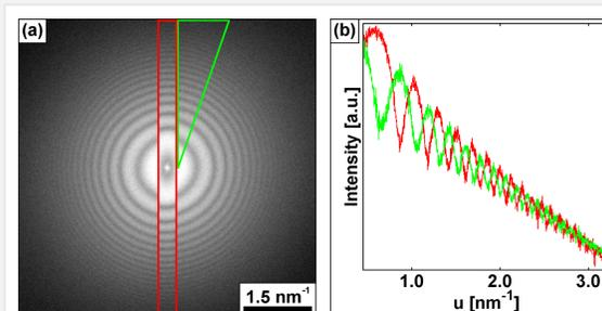
Fig. 5: Application of a ZAC-film-based Hilbert PP on an aC test object. (a) Diffractogram of a phase-contrast image of an aC test object. Vertical red lines mark the cut-on frequency given by the PP edge. (b) Azimuthally averaged intensity profiles taken in the red and green regions of (a).
