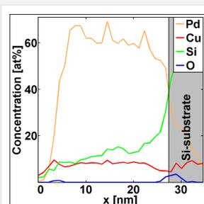
Fig. 4: Chemical composition of the PCS-alloy derived from an EDXS line profile.
