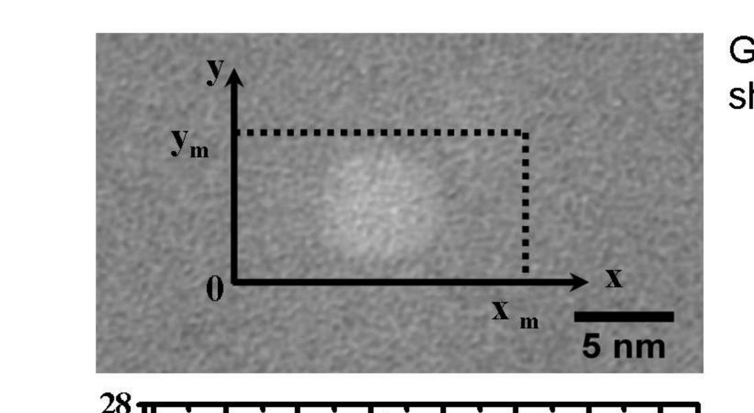
Gray-scale coded reconstructed phase shift for a gold cluster with D=6.9 nm
