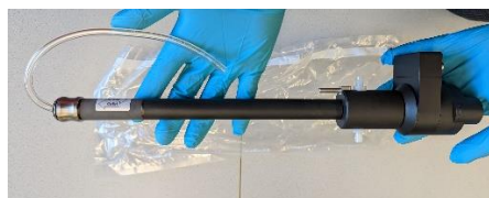
Fig.2: In-situ single tilt heating and straining holder
